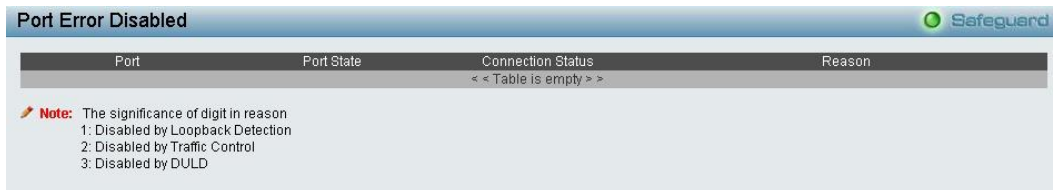
Figure 5.21 – System > Port Configuration > Port Error Disabled
