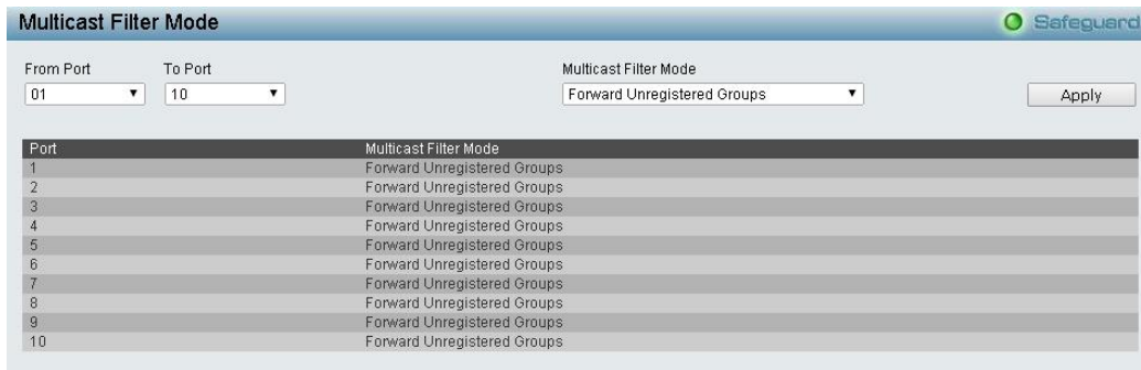
Figure4.78 - Configuration > Multicast Forwarding & Filter > Multicast Filter Mode
